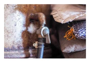
**STEP 1 –** Open the kerosene tank valve, turning the knob vertical.
