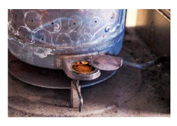
**STEP 4** – Open the small cover to the ignition hole, light a match, and put the burning end of the match inside the ignition hole, up against the nozzle to the right of the entrance, inside the stove.
