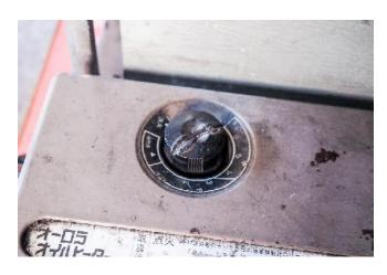
**STEP 3** – Turn the dial to 1. This will cause a very small amount of kerosene to start leaking into the stove.
